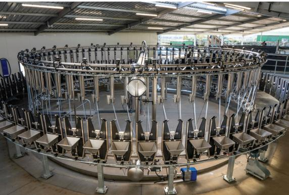
Constructed from stainless steel, the system is built for longevity - a key point of difference when compared to other sheep rotary systems. And for animal comfort, rubber mats are fitted to the deck for the sheep to stand on during milking, which also reduces noise and stress for both the animals and the operator. The internal platform also means the operator is standing inside the rotary so they can easily observe all of the sheep, all of the time.
